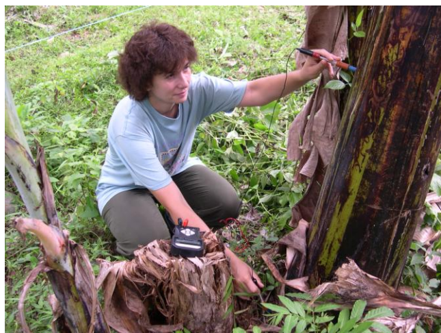
Fig. 5 Measurement of electrical potential between soil and banana plant in Philippines using Landmapper ERM-02.
