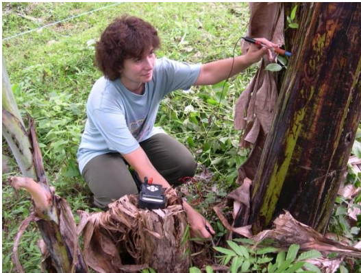
Fig 5. Measurement of electrical potential between soil and banana plant in the Philippines using Landmapper ERM-02.
